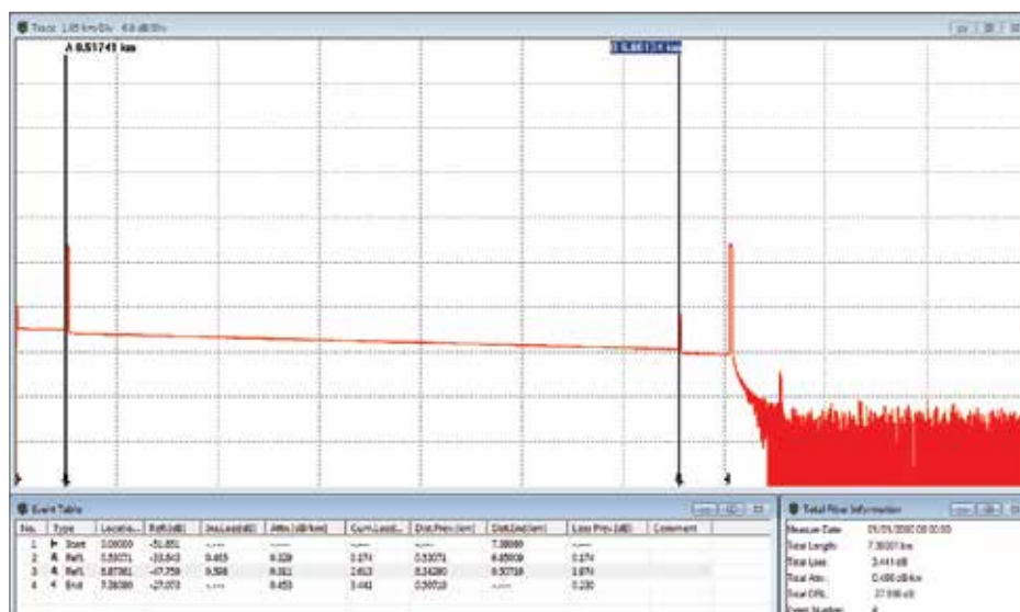
OTDR trace with LC-500 at start & end of Fibre under Test. Enables accurate measurement of end connectors.
