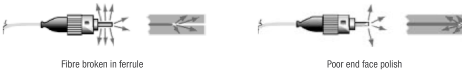
Fibre broken in ferrule
