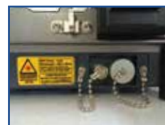
Power Meter and Fault Locator
