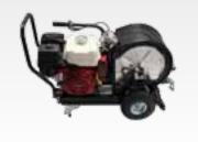
The easy removable cable drum provides enough space for 1100 m of cable with  $\emptyset$  4mm. For  $\emptyset$  5 mm steel cable the capacity amounts to about 700 m. We recommend a steel cable of  $\emptyset$  6 mm, to ensure a double safety for horizontal pulls. The capacity for this diameter amounts to 500m.
