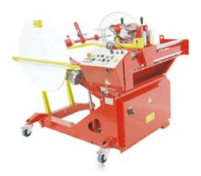
It is not always feasible to store or transport cables in rings. To allow for **simple**, **safe and fast recoiling** from one cable drum to another Katimex can offer a range of **stationary** or **mobile** drum winding machines.
