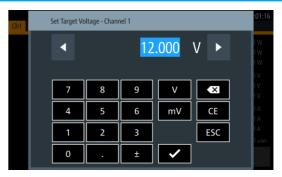
The large capacitive touchscreen is the central operating element on the R&S®NGM200. Lightly tapping a numerical value will display a virtual keyboard to enter the desired value. Alternatively, the rotary knob can be used to set voltage and current values as well as limits for the various protection functions.
