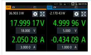
A resolution of up to 6½ digits is perfect for characterizing DUTs that have low power consumption in standby mode and high current in full load operation.
