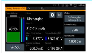
Capacity, open circuit voltage (Voc) and equivalent series resistance (ESR) are important battery characteristics that depend on the battery's state of charge (SoC). The optional R&S<sup>\*</sup>NGM-K106 battery simulator allows users to simulate the battery behavior under different charging conditions, e.g. when powering a DUT.
