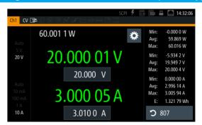
The large capacitive touchscreen is the central operating element on the R&S\*NGM200. The very high resolution of 800 x 480 pixel makes it easy to read voltage and current values even from a distance. Information such as power values and statistics can be displayed in addition. Icons indcate the status of selected protection and special functions.
