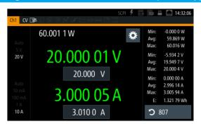
The large capacitive touchscreen is the central operating element on the R&S\*NGM200. The very high resolution of 800 x 480 pixel makes it easy to read voltage and current values even from a distance. Information such as power values and statistics can be displayed in addition. Icons indicate the status of selected protection and special functions.
