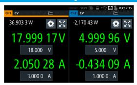
A resolution of up to 6½ digits is perfect for characterizing DUTs that have low power consumption in standby mode and high current in full load operation.
