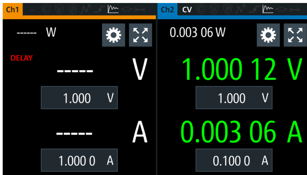
Figure 6-8: Delay text at channel display area
