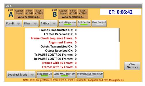
**Clear Statistics** – Press this button to Clear all the Port-B statistics and reset the elapsed time (ET) to zero.
