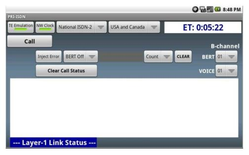
When the PRI circuit is connected this window is CURRENT Layer-1 STATUS and should say Layer-1 LINK ACTIVE. If LOSS of Signal is displayed please check cable connections.
