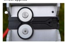
For micro cable size 3.0 - 4.5 mm NanoFlow MAX adaptor plates and MAX steel wheel applies.
