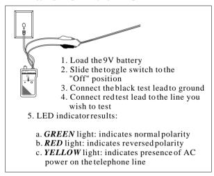
Note: If a ground is not available, you may try to switch the test leads around to different wires within the pair.
