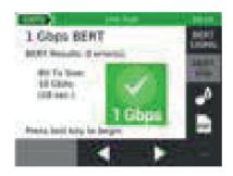
The BER Test will allow you to manually perform a Bit Error Rate Test without regard to TIA wiring specifications such as length maximum and pinout. This will allow you to identify if a cable can support 100Mbps or 1Gbps using up to 250 Gigabytes of data.
