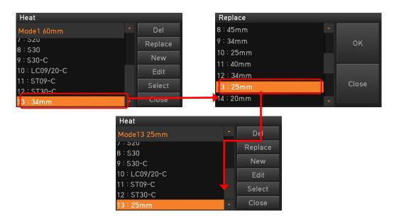
The mode from No 1 to 12 can't be replaced.
