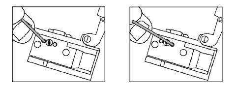
ii. Rotate the cleaver blade just 1 step using the cotton swab. (16 steps blade)
