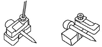
iii. Remove the electrode block and take out the used electrode.
