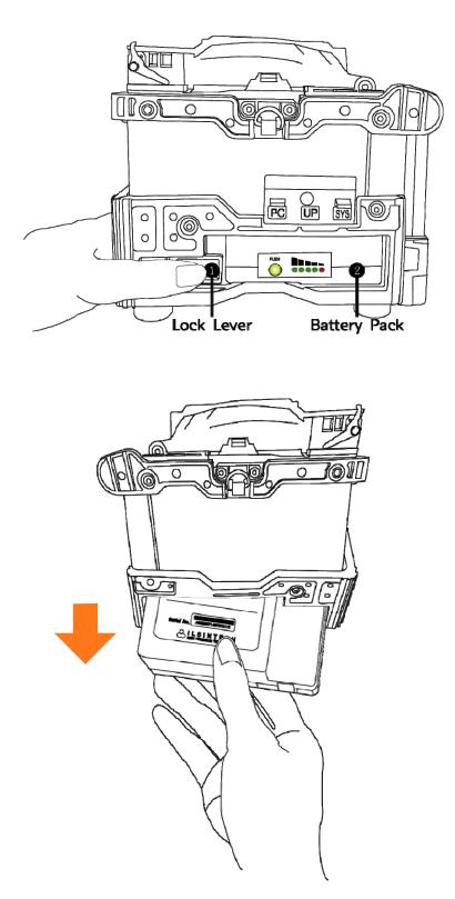
Please make sure the power is off before removing the battery. Remove the battery by releasing lock lever.
