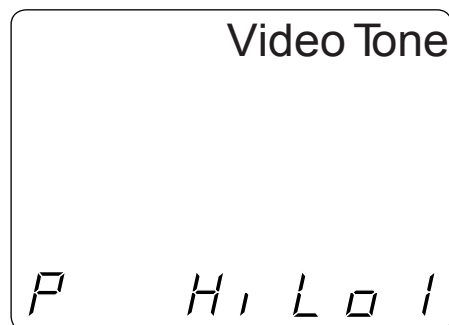
Figure 12. Video Cable Test with Pin Selected
