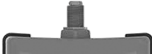
Figure 6. F-Connector on Main Tester
