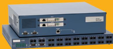
OptiView™ Link Analyzer and an 8 port in-line fiber tap.
